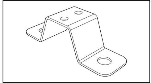
When connecting using a 10 sq. mm internal section cable, the existing clamp must be replaced with the one supplied in order to ensure that the cable is secured correctly.
