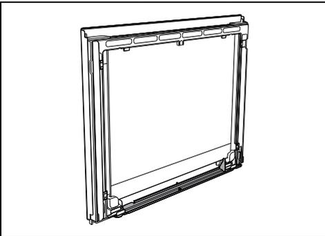
4. Place the internal glass panel back onto the brackets after cleaning. Make sure that you centre it and then insert the 4 pins firmly into their housings on the door with the help of
