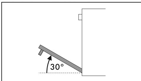
3. To reassemble the door, put the hinges in the relevant slots in the oven, making sure that grooved sections **A** are resting completely in the slots.
