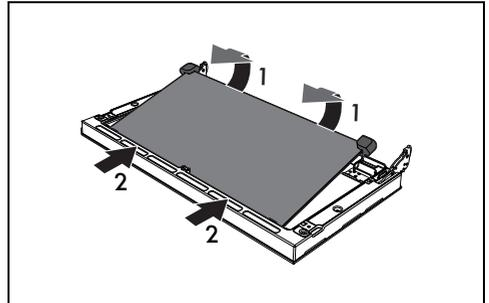
4. Replace the intermediate glass panels after cleaning.
