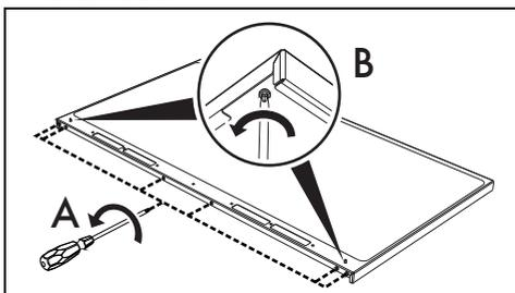
2. Place the upstand on the hob. Align the 6 bottom slots of the upstand with the 6 screws on the back of the hob that were previously loosened.
