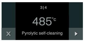
A signal sounds once the pyrolytic self-cleaning function has ended. A message appears in the display. Once the appliance has cooled down, wipe out the ash that has been left behind in the cooking compartment with a damp cloth.
