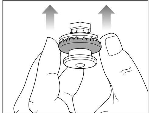
■ After cleaning, push the top heat/grill element back up using the outer ring of the pressure cap. Make sure the pressure cap engages correctly.
