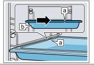
To place the accessory at shelf positions with pullout rails, pull out the pull-out rails.
