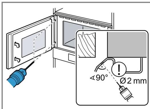
Cover the door hinges. Use a wood drill with a 2 mm diameter.
