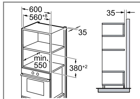
Do not fit the appliance too high up; it must be possible for accessories to be removed easily. Fit the feet.
