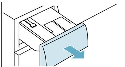
3. Press down the insert and remove the drawer completely.
