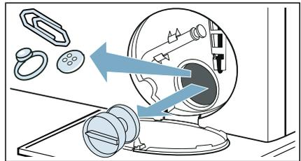
5. Refit and screw on the pump cover. The handle must be in a vertical position.
