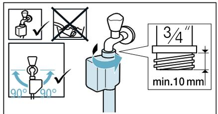
**Tip:** Connect also an external water filter (depending on the model) between water supply hose and tap. The filter filters dirt particles out of the water.
