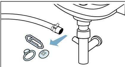
4. Re-attach the drain hose and secure the connection point using the hose clamp.
