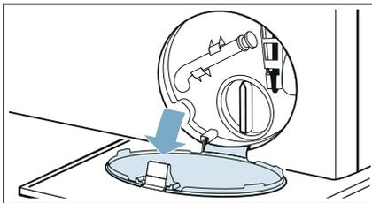
3. Take the drain hose out of the retainer. Remove the sealing cap and pour the water out into a suitable container. Replace the sealing cap and place the drain hose back in the retainer.
