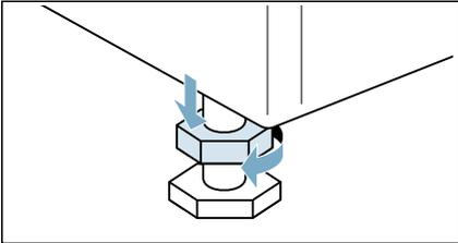
2. Check the alignment of the appliance with a spirit level, and adjust it if necessary. Change the height by turning the appliance feet. All four appliance feet must stand firmly on the ground.
