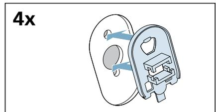
4. Lock the covers firmly in place by applying pressure to the snap-in hooks.
