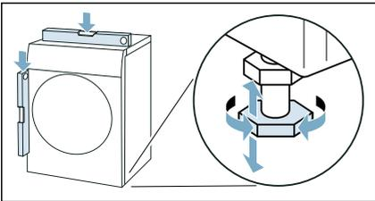
3. Tighten the lock nut against the housing. In doing so, hold the foot tight and do not adjust its height. The lock nuts on all four appliance feet must be screwed tightly against the housing.
