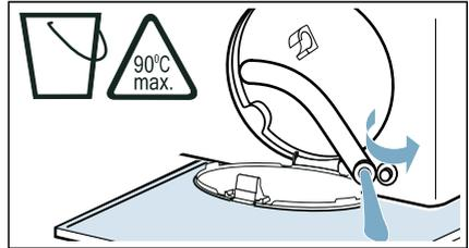
4. Carefully unscrew the pump cover; residual water may leak out. Clean the interior, pump cover thread and pump housing. The impeller in the drain pump must be able to rotate.
