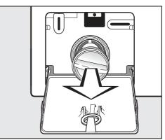
Remove the drain filter completely.
