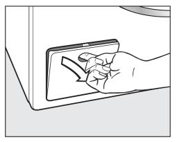
Open the drain pump access panel.
