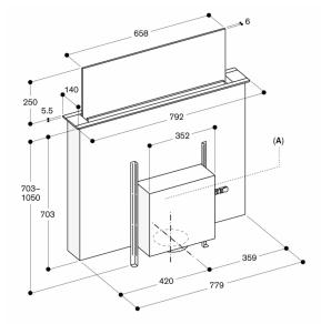
A: Flexible installation of the fan unit at the front, at the back or at a distance from the appliance (installation kit required - max. distance 3 m)
