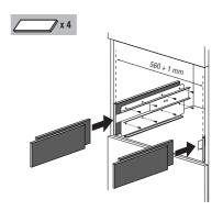
If necessary, correct alignment of the appliance by positioning the spacers supplied under or at the sides of the support.
