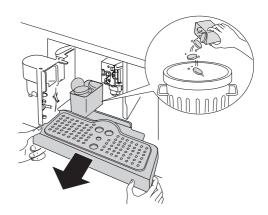
When cleaning, **always extract the drip tray completely** to avoid it falling when the grounds container is removed.
