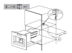
Fix the power cable with the clip to avoid it tangling when the appliance is inserted or extracted.
