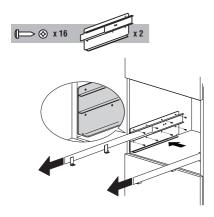
Position the rails on the sides of the cabinet as shown in the figure.
