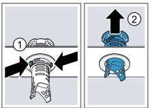
5. Clean the filter elements under running water. Carefully clean the rim of dirt between the coarse and the fine filter.
