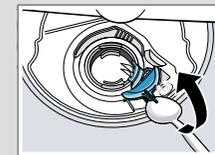
5. Lift the pump cover inwards at an angle and remove.
