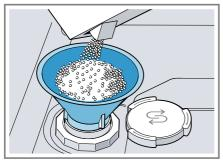
Fill the dispenser right up with special salt. The water in the dispenser is displaced and forced out.
