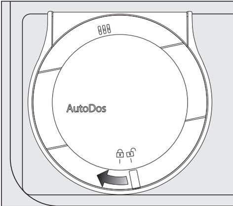
The detergent powder must be dry so that it does not clump together. Do not fill the AutoDos with any type of fluid.
