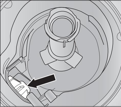
The drain pump (see arrow) is underneath the cover.
