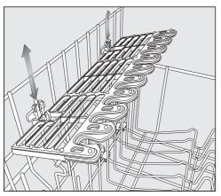
Slide the glass rack to the desired height until the catches click into place at the top or the bottom. The MultiClips enable you to fasten light items such as those made from plastic onto the glass holder.
