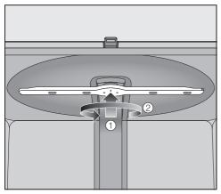
Push the upper spray arm upwards 1 to engage the inner ratchet. Then unscrew the spray arm by rotating the screw connection anti-clockwise 2.
