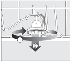
Rotate the screw connection of the middle spray arm clockwise 1 and remove the spray arm 2.
