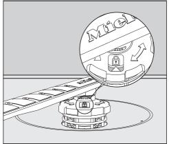
■ Rotate the screw connection clockwise until the arrow in the viewing window points to the lock symbol ⊕.
