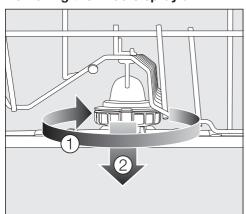
■ Rotate the screw connection of the middle spray arm clockwise ① and remove the spray arm ②.
