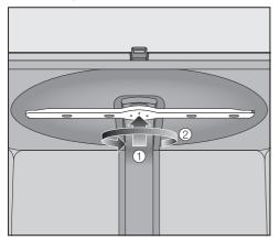
■ Push the upper spray arm upwards ① to engage the inner ratchet. Then unscrew the spray arm by rotating the screw connection anti-clockwise ②.
