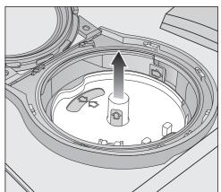
■ Pull the PowerDisk holder upwards by the yellow tabs and remove it. When doing so, do not pull on the side tab.
