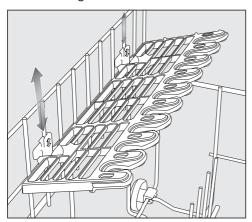
■ Slide the glass holder to the desired height until the catches click into place at the top or the bottom.
