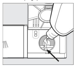
Fill with rinse aid until the filling level indicator (arrow) changes to a dark colour while the door is horizontally open.
