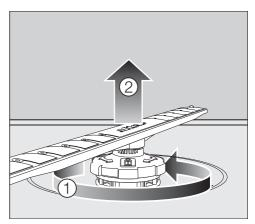
■ Rotate the screw connection of the lower spray arm anti-clockwise ① and pull the spray arm upwards to remove ②.
