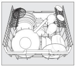
■ Place larger and heavier items such as plates, serving platters, pots, bowls and woks in the lower basket. Glasses, cups and small plates can also be placed in the lower basket.
