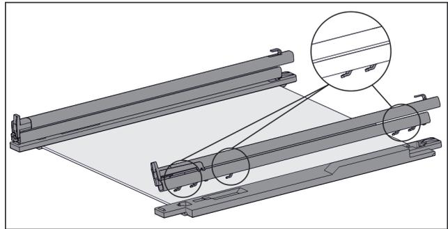
*Fig. 126 Glass shelf with rails and retaining parts*
