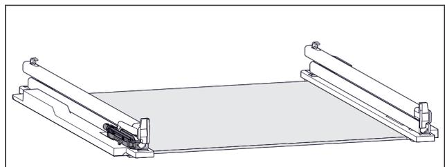
*Fig. 129 Damping mechanism*
