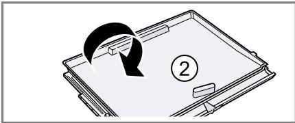
3. Press the fastenings for the lower cover outwards.
