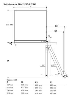
In the drawing, a unit front thickness of 19 mm and a Gaggenau unit handle of 49 mm were taken as a basis.
