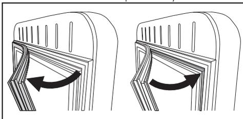
1. Remove the seal by pulling it out of its housing.
