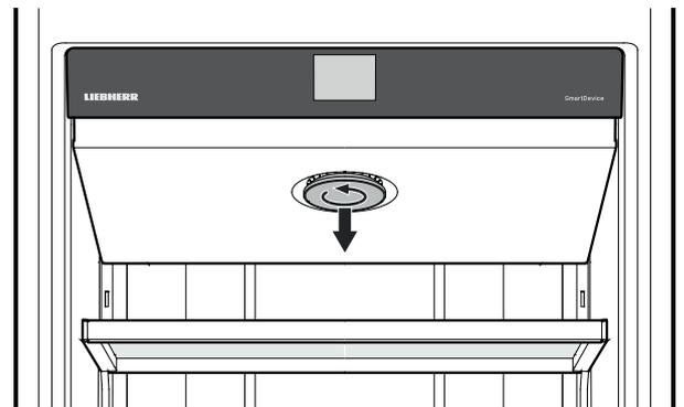
Turn the cover anticlockwise and remove it.
