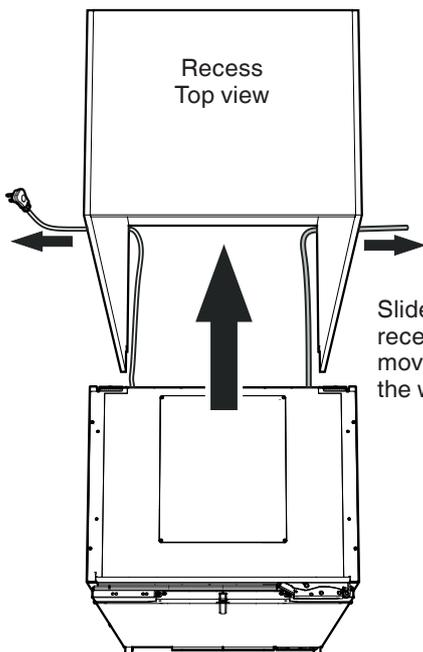
Slide the appliance into the recess. To avoid damage, move the mains cable and the water line at once.
