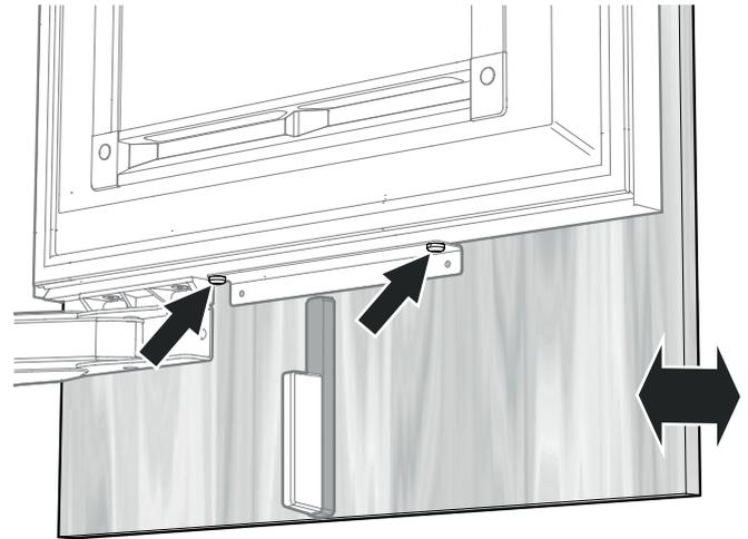
Secure the panel through the bottom attachment bracket with two 4 x 14 screws.
