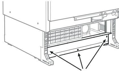
The steel plate can be removed to facilitate connecting the water hose.
