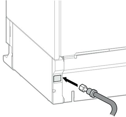
Pull the water line through from the rear to the front.
