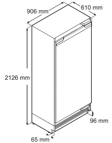
Stated minimum height dimensions include when the adjustable feet are fully inserted. Width will increase by 6.5 mm when mounting strips are installed.
