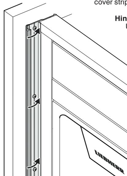
Push the mounting strip upwards.
