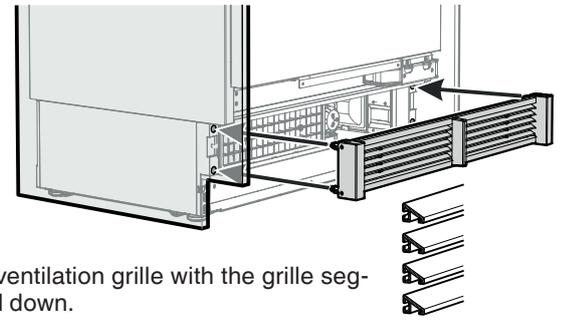
Mount the ventilation grille with the grille segments tilted down.
