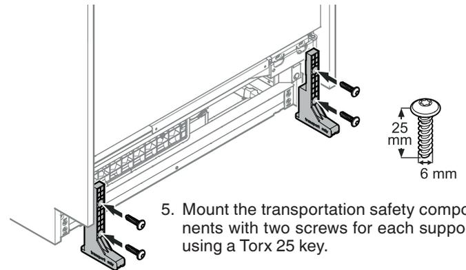
5. Mount the transportation safety components with two screws for each support using a Torx 25 key.
