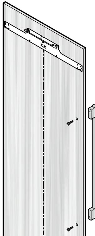
Only use countersunk screws for handle mounting.
