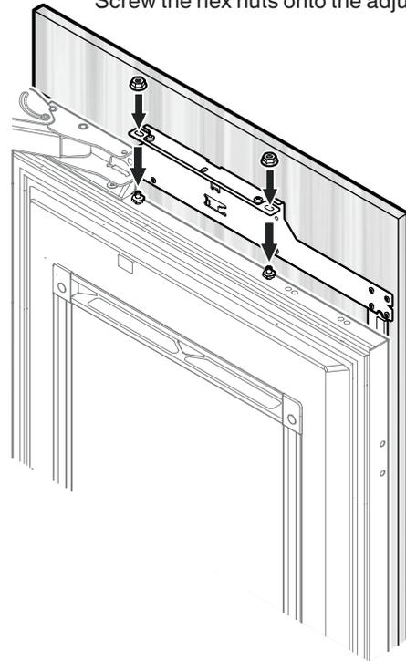
Close the door and check the position of the door panel.
