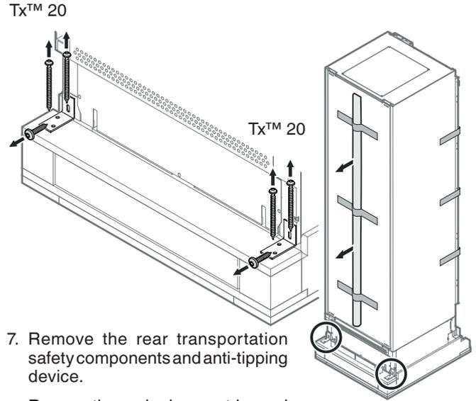
7. Remove the rear transportation safety components and anti-tipping device.
