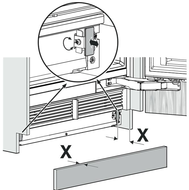
Remove the backing foil and affix the plinth panel.
