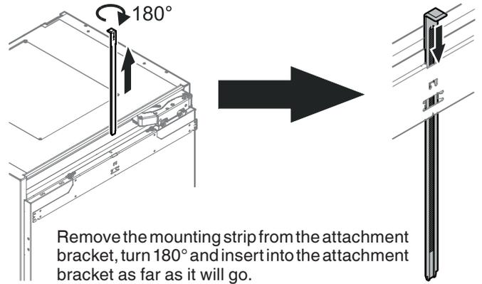
Remove the mounting strip from the attachment bracket, turn 180° and insert into the attachment bracket as far as it will go.
