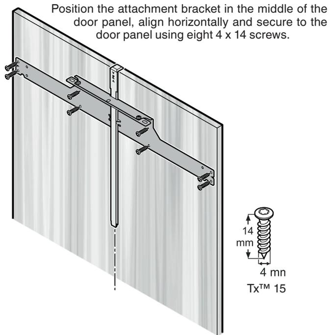
Position the attachment bracket in the middle of the door panel, align horizontally and secure to the door panel using eight 4 x 14 screws.
