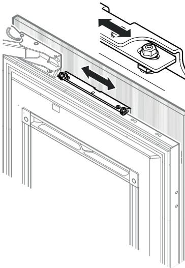
Align the panel horizontally with the long slots in the attachment bracket.
