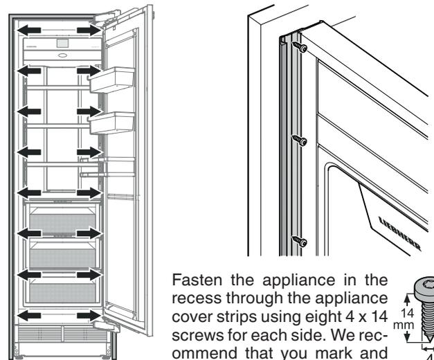
Fasten the appliance in the recess through the appliance cover strips using eight 4 x 14 screws for each side. We recommend that you mark and pre-drill the hole positions in the strip.
