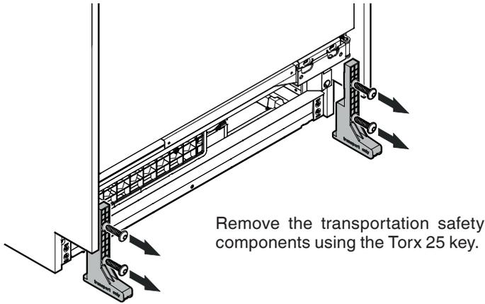
Remove the transportation safety components using the Torx 25 key.
