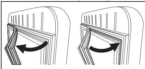
1. Remove the seal by pulling it out of its housing.
